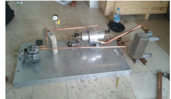
Steam turbine at Al Balqa
