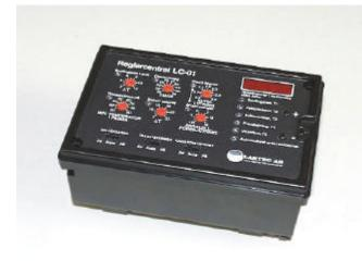
• An example of an integrated controller for solar combisystems, courtesy Lartec AB, Sweden
