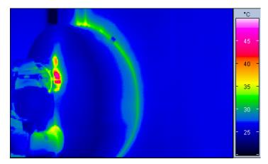
• Investigation on a hot water tank by means of infrared thermography. The heat losses are minimised thanks to optimal integration of an auxiliary heater with the help of a new insulating material, SOLVIS, Germany
