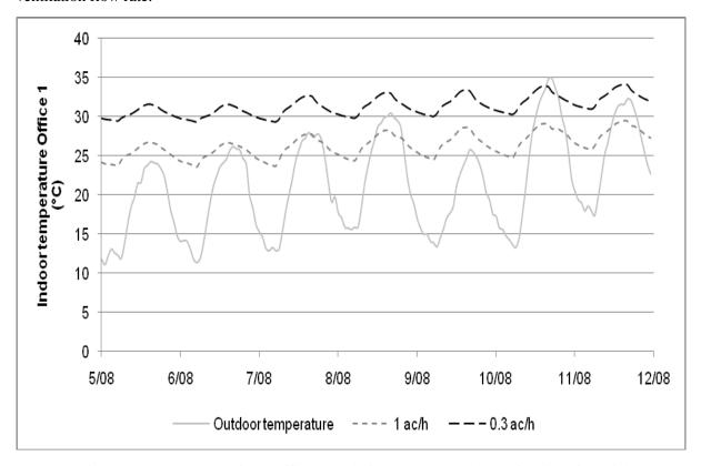
Fig. 4. Temperature curve for an office room during a summer week as a function of the night ventilation flow rate.
