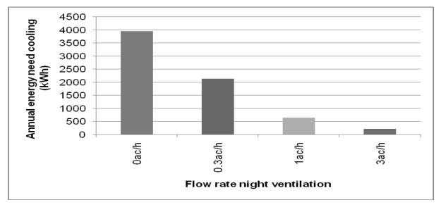
Fig. 3. Annual energy need for cooling of the first floor as a function of the night ventilation flow rate.
