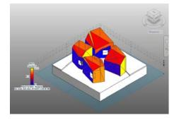
Figure 3: Project Vasari can present various solar radiation options: cumulative, average mean of hourly values, and peak maximum value in [kWh/m²/year]. Output such as this can help improve communication with engineer and solar consultant and can lead to joint decision making regarding solar strategies. In order to assist communication between architect and client such results could be transferred into potential energy savings or potential financial savings.
