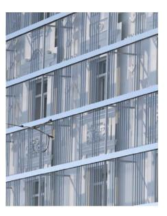
Figure 5: Visualization of proposal for evacuated tube collectors in front of listed building façade in Graz, Austria. Source: Institute of Architectural Typologies, Graz Technical University
