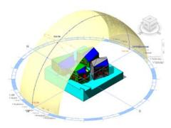
Figure 1: Revit: A sun path shows how natural light projects shadows onto the buildings due to neighboring buildings and terrain
