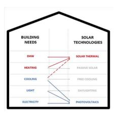
Figure 1: Solar technologies covering different building energy needs (EPFL/LESO-PB)
