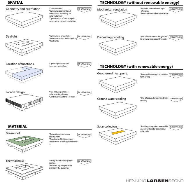
Figure 4: Consequences of different design parameters on the energy use of a
