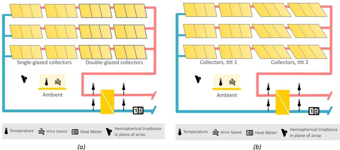
**Figure 16.** Examples of collector fields composed of different collector models within each row: (a) combination of single- and double-glazed collectors; (b) combination of collectors with different tilt angles.
