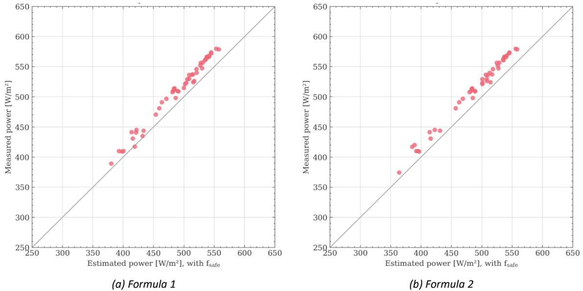
**Figure 53.** Effect of Power Check Formula: (a) Formula 1 (50 valid data records) and (b) Formula 2 (47 valid data records). Data: May 2017. Details: Power Check Formula 1 and 2, data averaging as in ISO 24194, wind considered,  $f_{\text{safe}} = 90\%$ . Numeric results in [Table 20](#): (a) Case 1a, (b) Case 1b.
