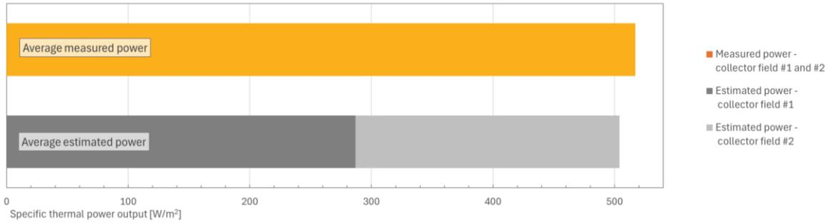
**Figure 10.** Proposed extension of Power Check to multiple collector fields: Comparison of average measured and estimated power output (for collector field #1 and #2) with the sum of the estimated power outputs for collector field #1 and #2.
