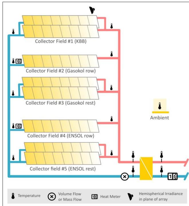
**Figure 58.** Measurement setup for Solar District Heating plant Mürzzuschlag. Heat meters are installed for the whole plant (primary side and secondary side) and in one row (“guarantee row”) of the Gasokol and ENSOL collector fields. The collector orientation (tilt, azimuth) is the same for all fields, therefore a single radiation sensor is sufficient.
