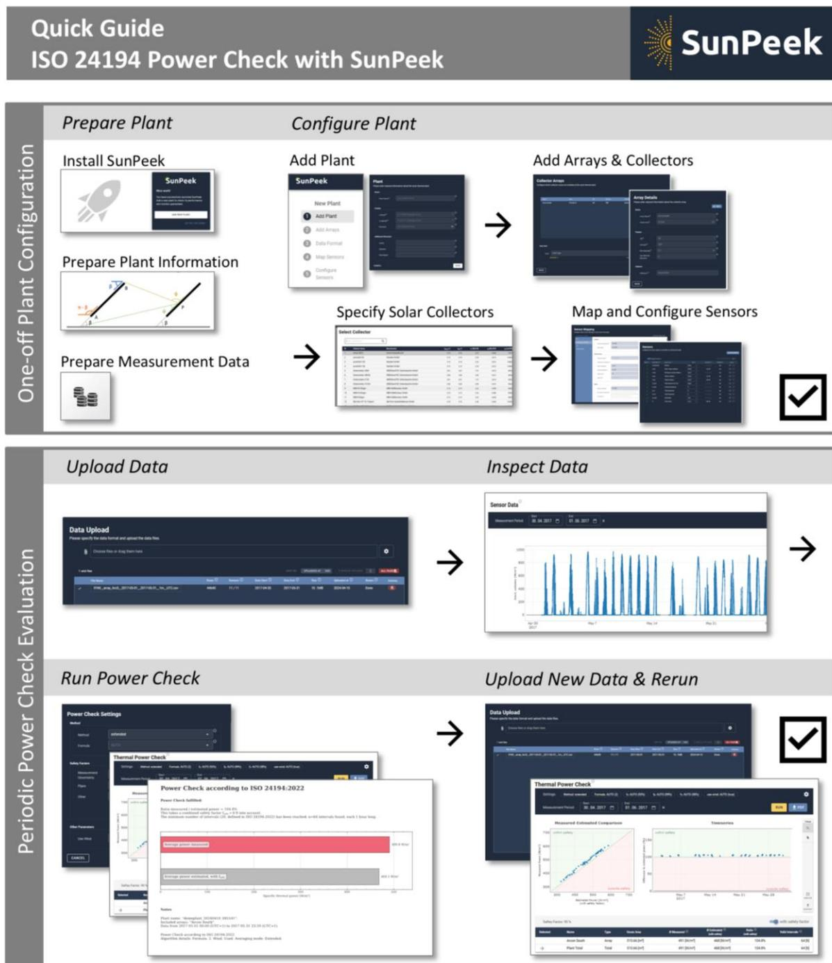
Figure 19. Quick Guide to ISO 24194 Power Check with SunPeek.
