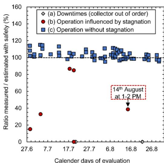
**Figure 61.** Influence of downtimes and stagnation events on Power Check results for a Solar District Heating plant with approximately 6000 m<sup>2</sup> collector area. The plot shows the measured-estimated power ratio for 1-hour intervals: a) data with downtimes (grey diamonds), b) data without downtimes, influenced by stagnation (red circles), and c) typical operation without stagnation (blue squares). Source: ISFH.
