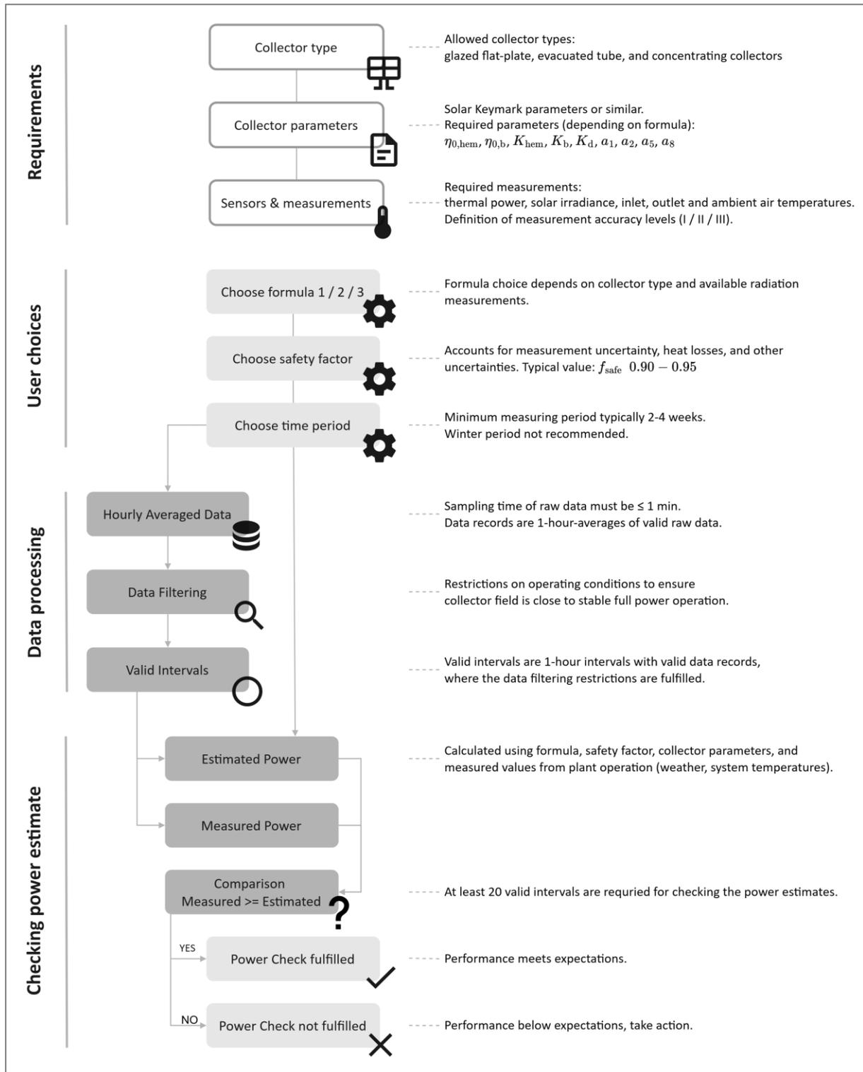
Figure 1. Step-by-step procedure of the ISO 24194 Power Check.
