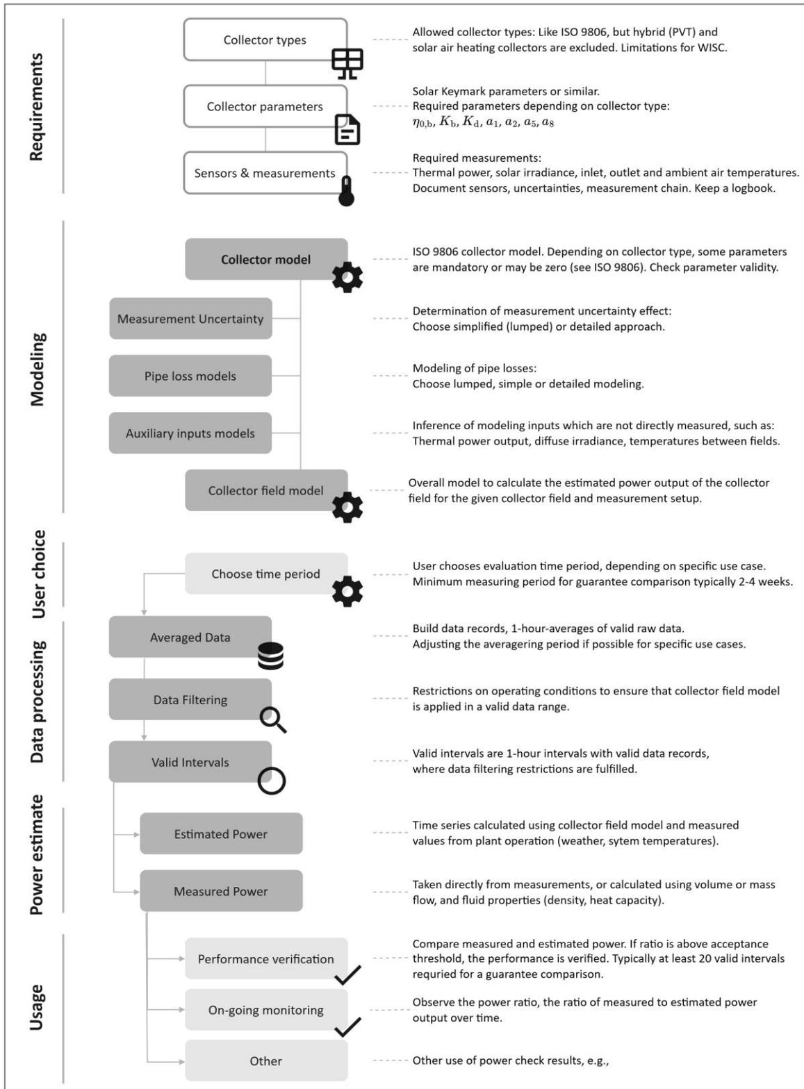
Figure 67. Step-by-step procedure of Harmonized Power Check framework.
