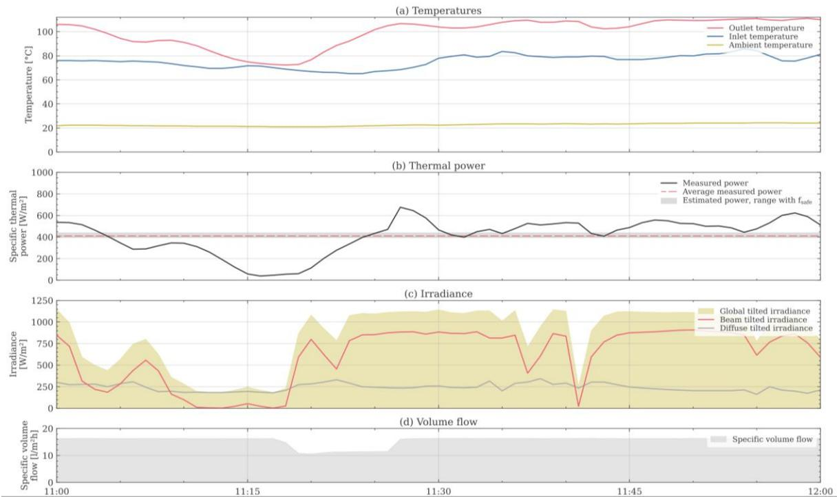
**Figure 49.** Time-series plot for an example valid data record: Subplot (a) shows collector field inlet / outlet and ambient temperatures, (b) measured and estimated power output, (c) hemispherical, beam, and diffuse irradiance, and (d) specific volume flow. Details: Formula 2, data averaging as in ISO 24194, wind considered,  $f_{safe} = 90\%$ .
