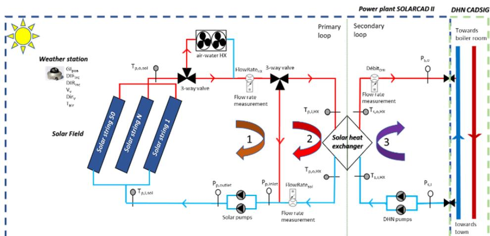
Figure 63. Simplified hydraulic flow diagram of the SolarCADII Solar District Heating plant, indicating sensor locations.
