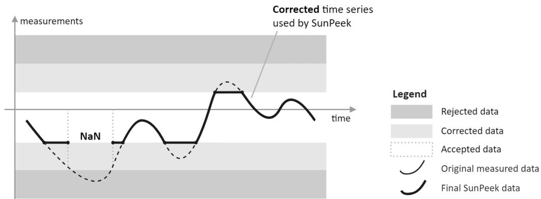
**Figure 39.** Data quality checks in SunPeek for treating gross errors. Values inside a “tolerance range” are corrected, values outside are set to NaN.
