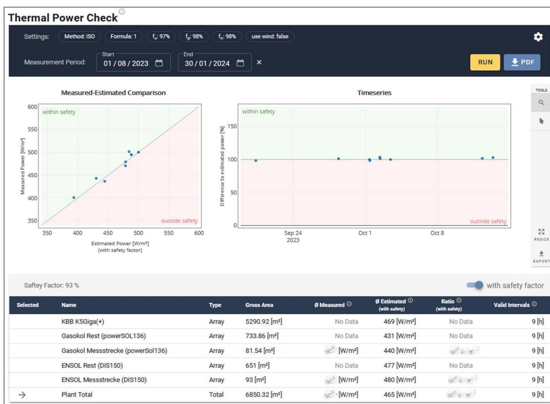
**Figure 60.** Screenshot of SunPeeK depicting Power Check results for Solar District Heating plant Müzzuschlag (measured results are anonymized). Using this setup, Power Check can be applied to the i) Gasokol guarantee row (measuring track), ii) ENSOL guarantee row (measuring track) and iii) total plant (selected in the Web-UI and graphically depicted).
