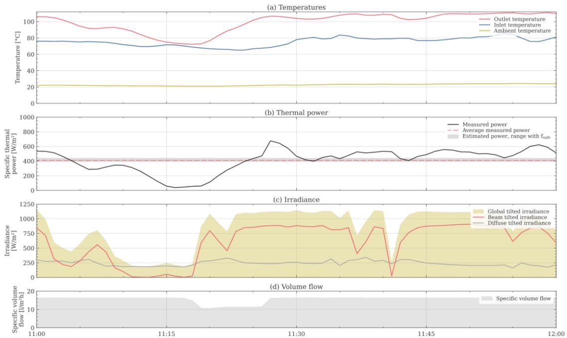
**Figure 18.** Data in a valid 1-hour interval showing a temporary dip in power output due to reduced irradiance. Such intervals would be ruled out by a minimum specific power output criterion used to detect stagnation.
