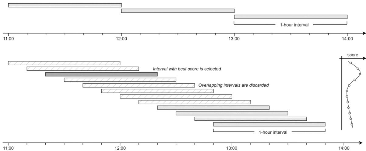
**Figure 6.** Comparison of Power Check averaging methods. The default method (top) is limited to intervals confined by full hours. The extended method (bottom) uses moving windows and selects intervals based on a score metric. Source: [28].
