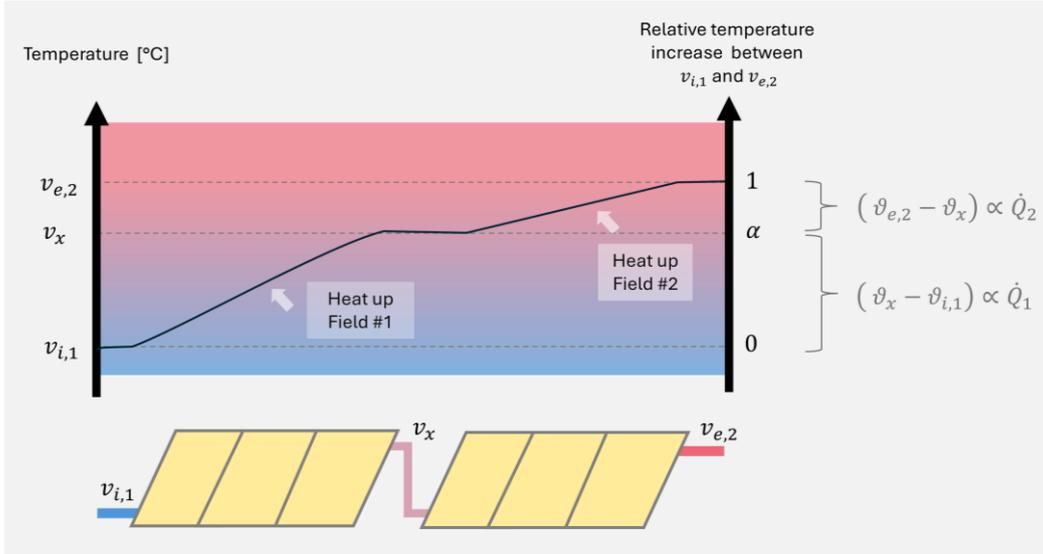
Figure 15. Illustration of inter-field temperature  $v_x$ .
