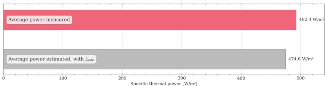
**Figure 46.** Overall Power Check results for the demo plant for full-year 2017: Measured and estimated specific power, averaged over all 270 valid data records. Average power ratio: 103.7% (Power Check fulfilled). Details: Formula 2, data averaging as in ISO 24194, wind speed considered,  $f_{safe} = 90\%$ .
