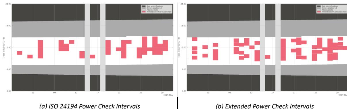
**Figure 52.** Comparison of valid intervals (data records) found with (a) ISO 24194 Power Check and (b) Extended Power Check. Data from May 2017. Details: Power Check Formula 2, wind considered,  $f_{\text{safe}}=90\%$ .
