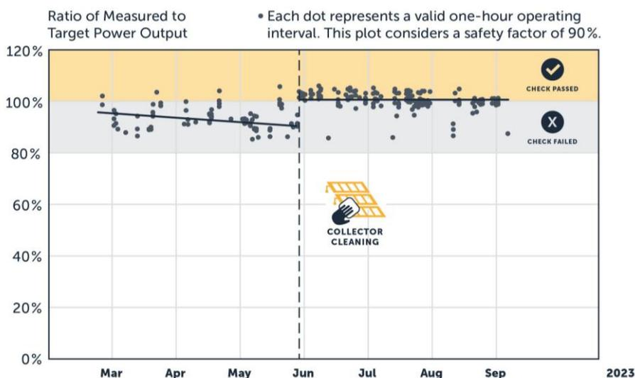
**Figure 57.** SunPeek screenshot, showing the measured-estimated power ratio over time. A pattern shift happens around Mid-June 2023, after collector cleaning. The figure shows real measurement data but has been graphically enhanced to better highlight the collector cleaning and pattern change.
