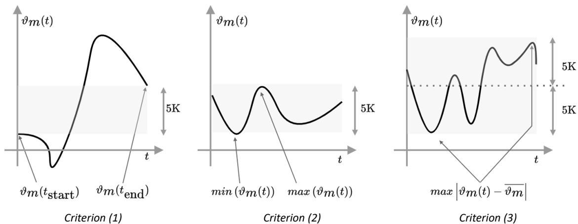
**Figure 3.** Data filtering criteria for mean collector temperature. Criterion (1) aims to avoid significant heat up or cool down phases, considering only the temperature at the start and end of the interval, but allowing arbitrarily large fluctuations within the interval. Criterion (2) aims to avoid significant temperature peaks or dips, considering all values within the interval. Criterion (3) targets significant temperature deviations compared to the mean temperature in the interval.
