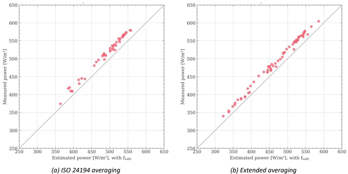
**Figure 54.** Effect of data averaging (see [Section B.1](#)): (a) Data averaging as in ISO 24194 (47 valid data records, average power ratio 104.9%), (b) Extended data averaging (64 valid data records, 104.8%). While numeric results are very similar, the Extended averaging covers a wider power range and finds more data records. Data: May 2017. Details: Power Check Formula 2, wind considered,  $f_{\text{safe}} = 90\%$ . Numeric results in [Table 20](#): (a) Case 2b, (b) Case 2c.
