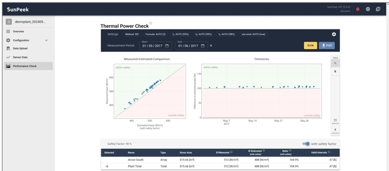
**Figure 35.** Screenshot of interactive graphical and tabular display of Power Check results. Each dot represents one valid data record (1-hour interval). The toggle on the bottom-right allows interactively switching the safety factor on or off.
