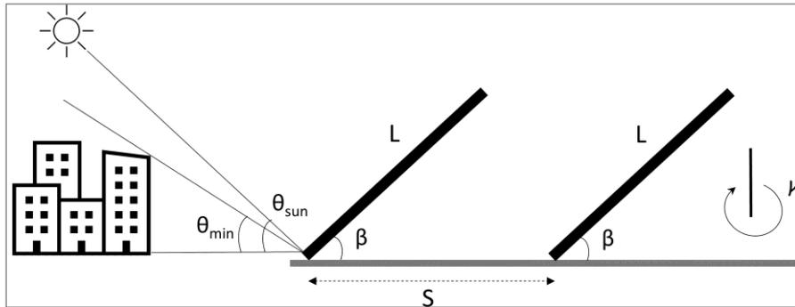
Figure 4. Collector field geometry with basic parameters and angle for external shading. In this figure the collector length ( $L$ ) runs from bottom to top as stated in ISO 9488:2022 [16], in contrast to Figure 1 in ISO 24194 where the collector width runs from bottom to top.
