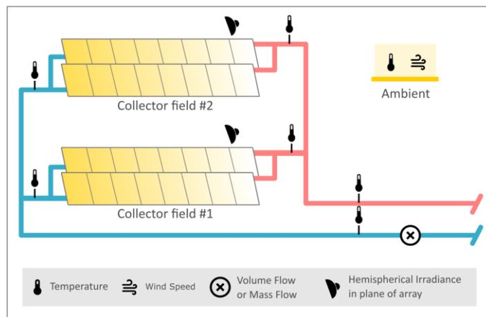
Figure 8. Example setup for a plant with two collector fields.
