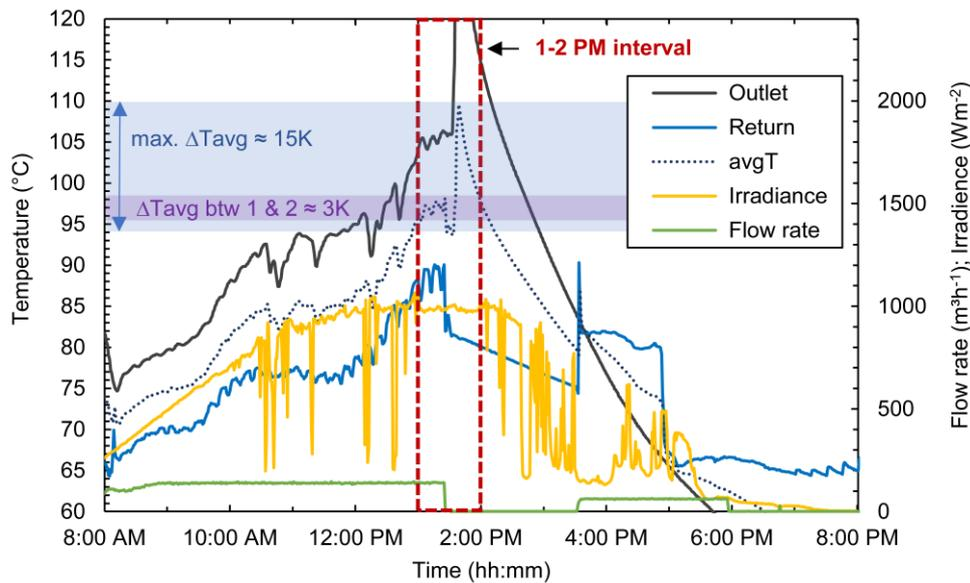
**Figure 17.** Impact of stagnation events on data selection of Power Check. The interval from 1–2 PM has a change in mean collector temperature of  $\approx 3$  K as the array cools down after reaching stagnation temperatures. This interval is a valid data record fulfilling all ISO 24194 criteria on operating conditions if the “change in collector mean temperature” criterion is interpreted as in [Figure 3 b](#), i.e.  $|\overline{d\vartheta_m/dt}| \leq 5$  K within an hour.
