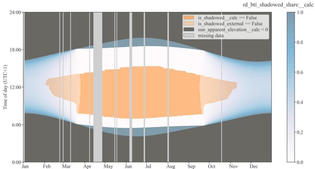
**Figure 44.** Collector field shading: Internal shading (calculated in SunPeak) and external shading (calculated with external tool) for the full demo plant period. Orange: Unshaded periods. Bright orange: Periods with no external shading. Color bar: fraction of row-to-row beam shading. Vertical grey lines: missing data. Source: [28].
