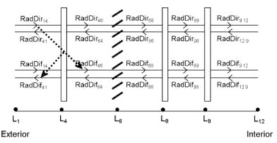
Figure 3. Schematic diagram of a four-flux model with four active layers. The dotted arrows mark a direct-diffuse transmission and reflexion of layer L4. [63].
