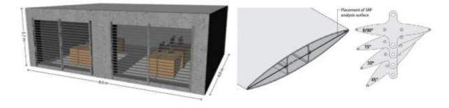
Figure 8. a) The original building geometry from the Best Test case 600 is an 8x6 meter room with two 3x2 meter windows facing southwards. b) Louvre-blade geometry and tilt angle illustration.
