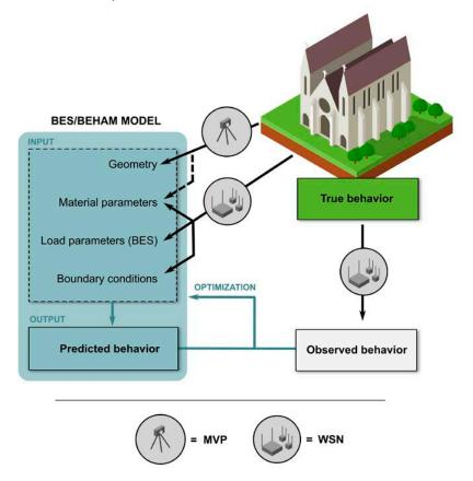
Figure 2. Complementarity of Multi-View Photogrammetry and Wireless Sensor Network to improve the hygrothermal modelling of heritage Buildings.
