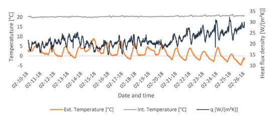
Figure 10. The hybrid WSN system makes it possible to monitor advanced variables remotely, such as the heat fluxes through walls.
