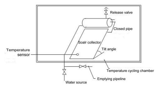
Figure 6 - Schematic for freeze resistance test apparatus for the solar system
