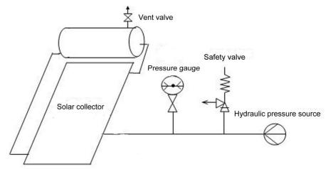
Figure 1 - Schematic for pressure resistance test for the solar system
