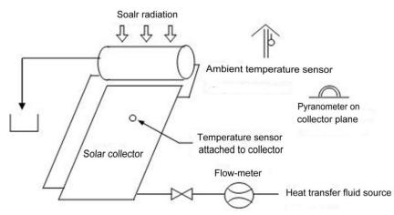
Figure 5 - Schematic for internal thermal shock test for the solar system
