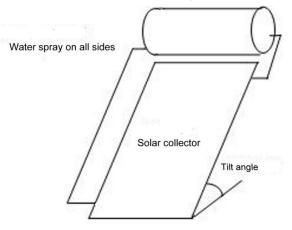
Figure 4 - Schematic for rain penetration test for the solar system
