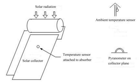
Figure 3 - Schematic for external thermal shock test for the solar system
