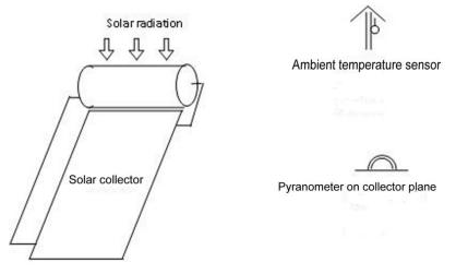
Figure 2 - Schematic for exposure test for the solar system
