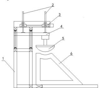
Figure 2 - Schematic diagram of support structure performance test bench
