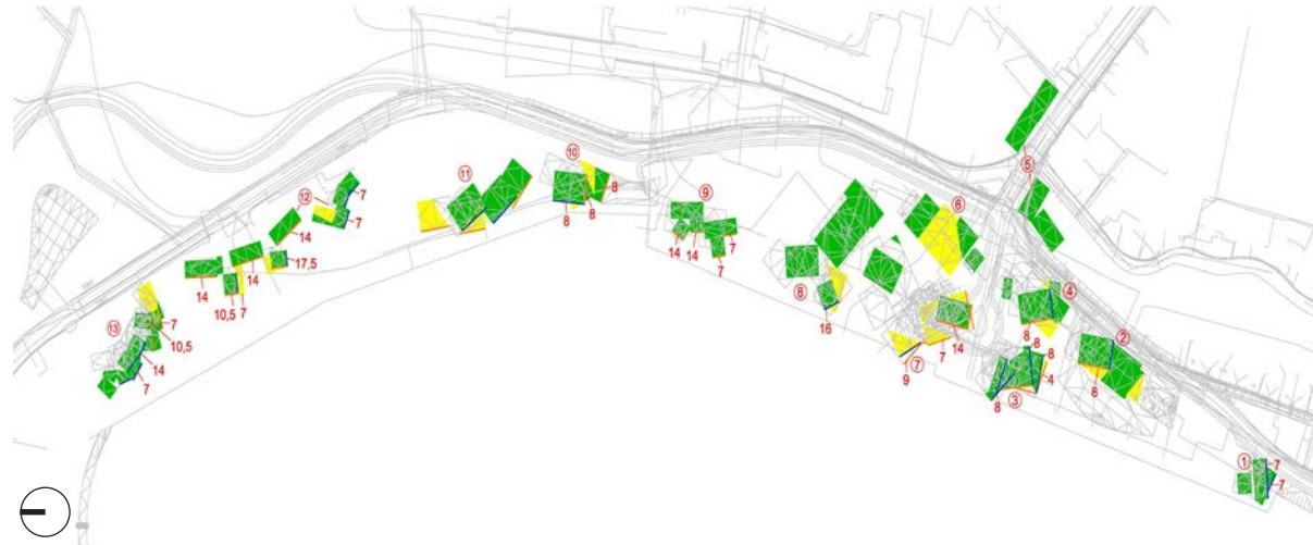
Figure 2 - Roof areas suitable for implementation of PV. Green marks roof areas with no shading. Yellow marks roof areas with shading 2 – 3 hours pr. day. In total 70 % of the roof area is suitable for implementation of PV. (Source: © Dansk Energi Management & Esbensen A/S)
