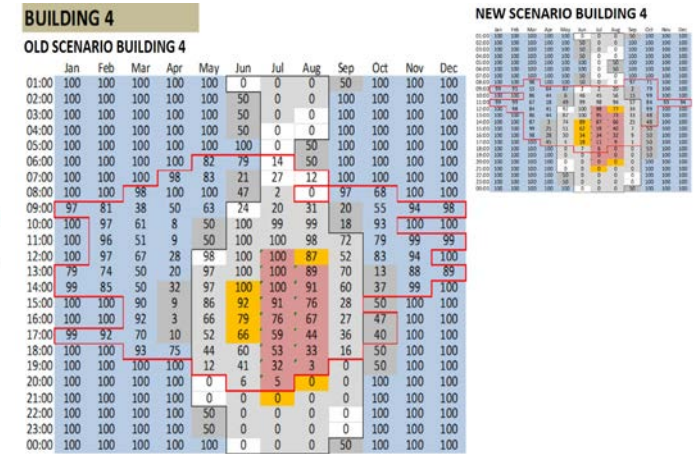
Figure 16 - Isopleth map with CBA bioclimatic chart zones in different colors. Black line identified the period where shade is necessary to prevent overheating; red line represent the average percentage of shading due to the surrounding buildings. (Source: © SUPSI)
