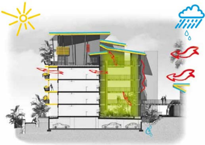
Figure 5 - The integrated passive bioclimatic measures ensure comfort for the buildings' occupants even in a high density development. (Source: © AP Architectures/2APMR)
