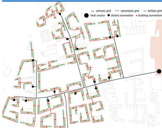
Figure 5 - System for a Local Heat Network at the primary research area (Source: TU Graz, Institute of Thermal Engineering: S. Grünewald)
