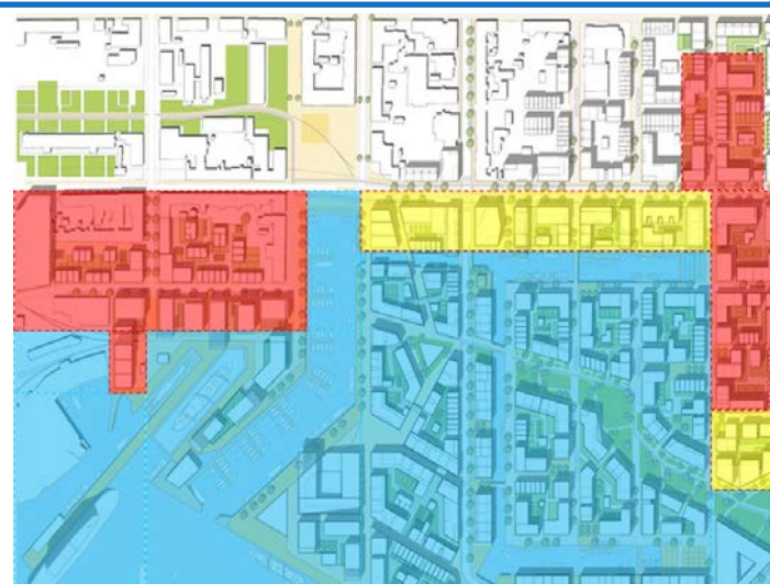
Figure 2 - Proposed heating supply, Blue: Heat pumps, Red: District heating, Yellow: Heat pumps or District heating (Source: © FredericiaC)
