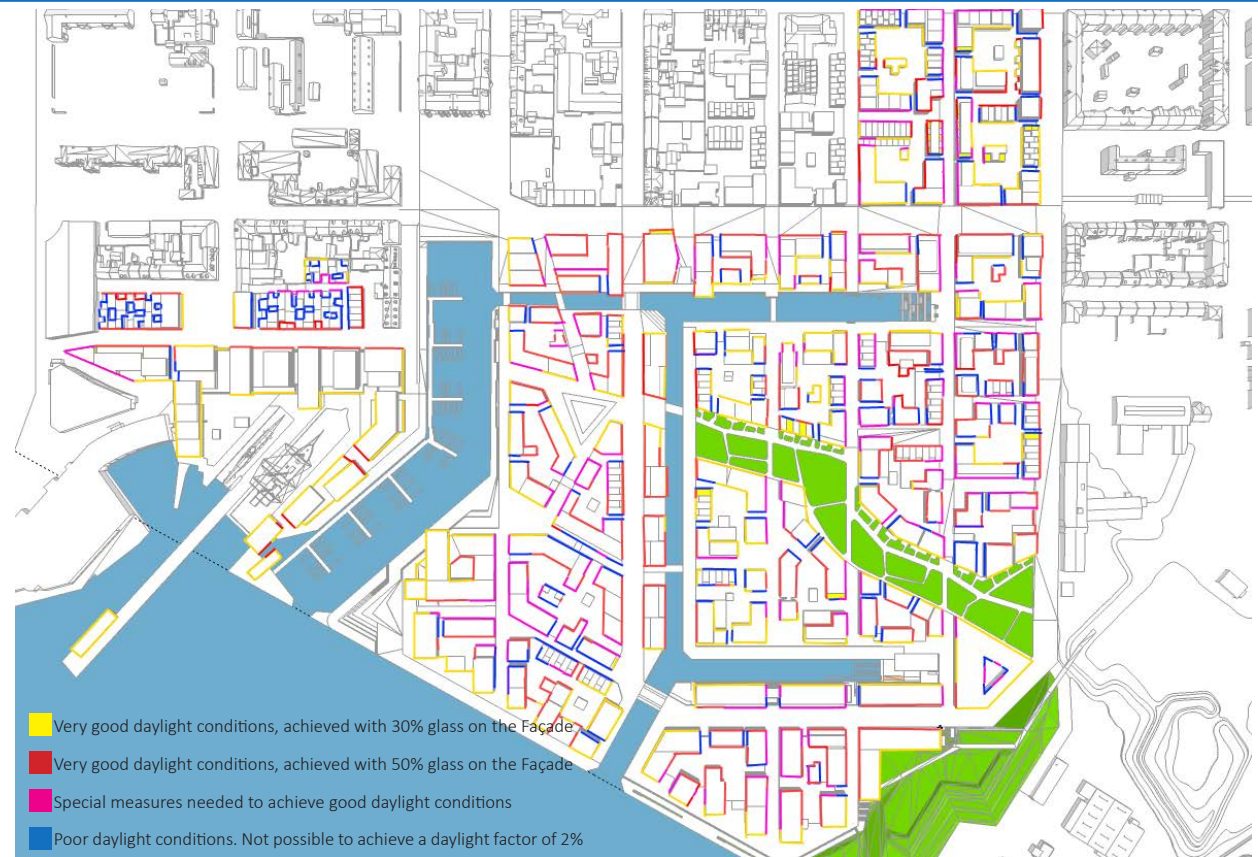
Figure 13 - Daylight levels on facades in the final development plan. (Source: © DEM & Esbensen A/S)
